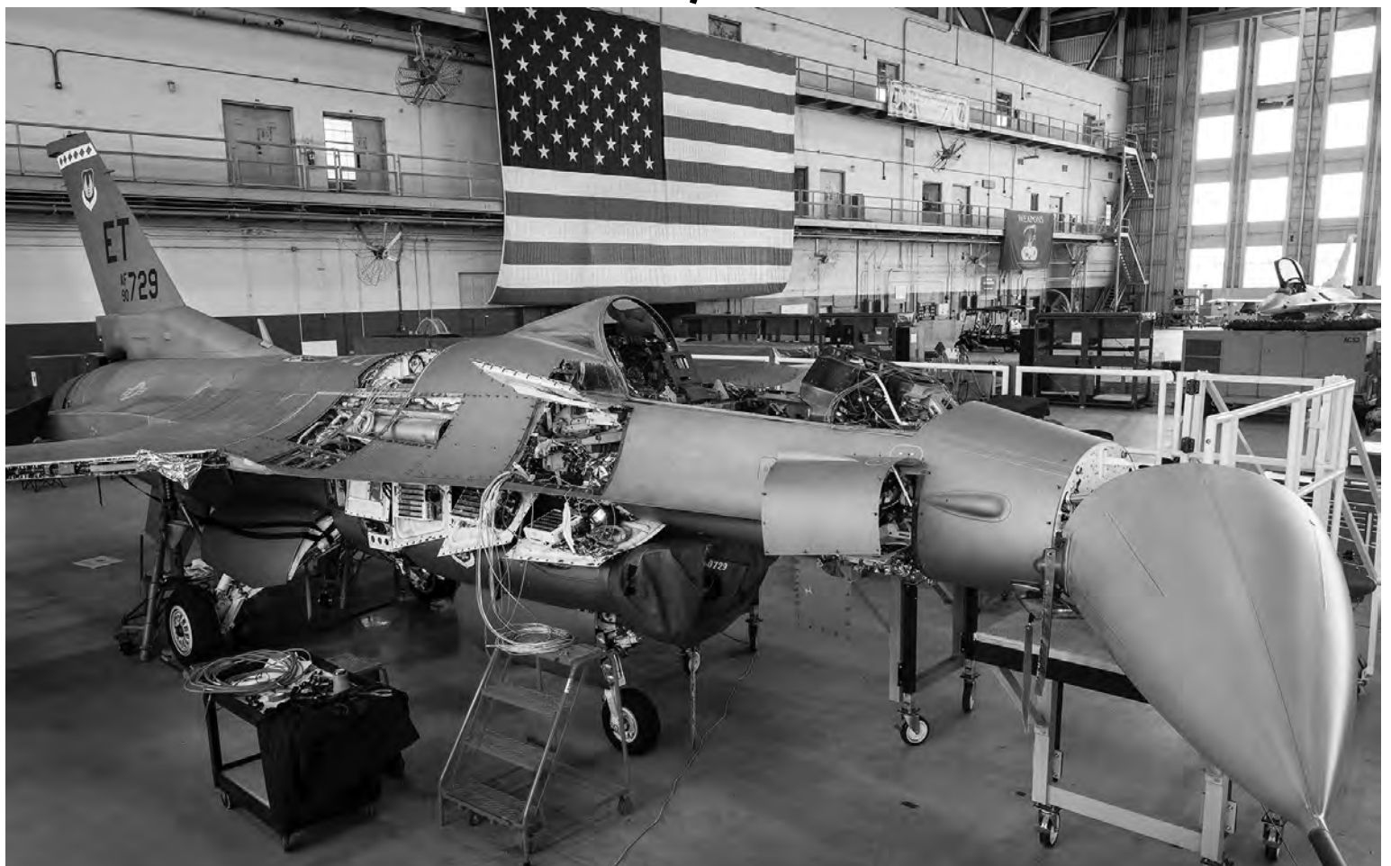
U.S. Air Force Photos by Samuel King Jr. An F-16 Fighting Falcon undergoes modifications as part of the Viper Experimentation and Next-gen Operations Model – Autonomy Flying Testbed program at Eglin Air Force Base, Florida. The changes include software, hardware and instrumentation that will allow the aircraft to fly autonomously.
