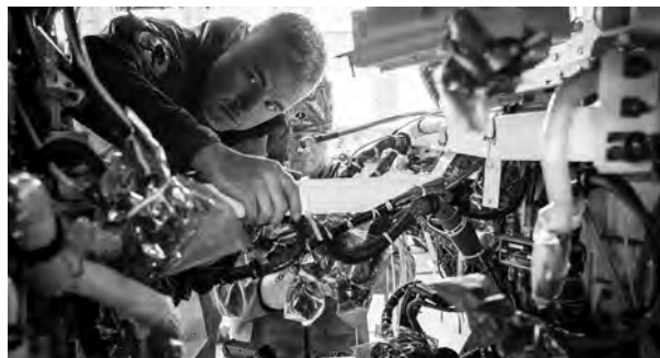
Chris Kiser, an aviation engineer, works on modifying an F-16 Fighting Falcon's wiring as part of Viper Experimentation and Next-gen Operations Model – Autonomy Flying Testbed program at Eglin Air Force Base, Florida. The changes include software, hardware and instrumentation that will allow the aircraft to fly autonomously.
